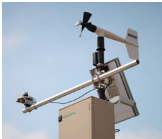
Environmental information is key to analysing and interpreting phenotypic data. Environmental stations closely monitor growing conditions within FieldScan.
